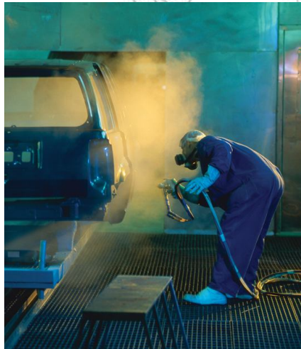
Figure 2.17 An electrostatic spray gun in use.
