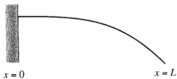
(b) cantilever beam: embedded at the left end, free at the right end
