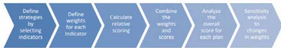
Figure 19. Schematic of steps within the analysis of plans in the FDMT basin planning application. Source: http://www.flooddroughtmonitor.com/home
