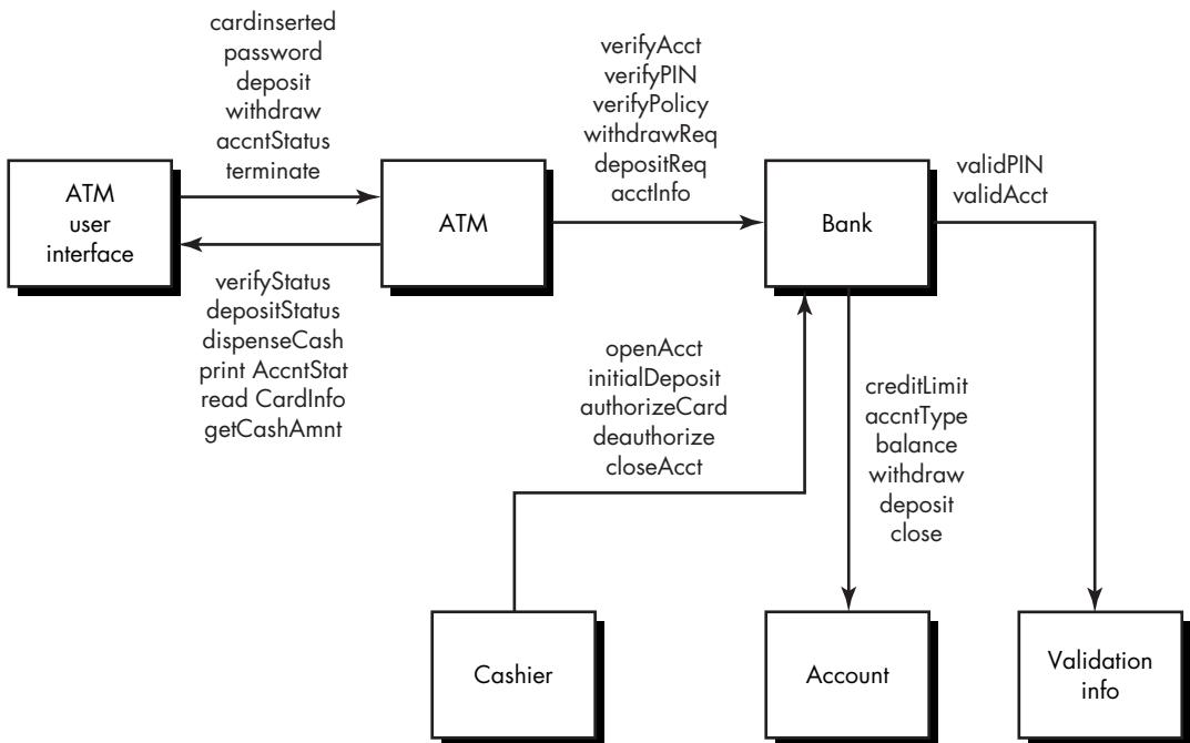
**FIGURE 23.2** Class collaboration diagram for banking application [KIR94]
