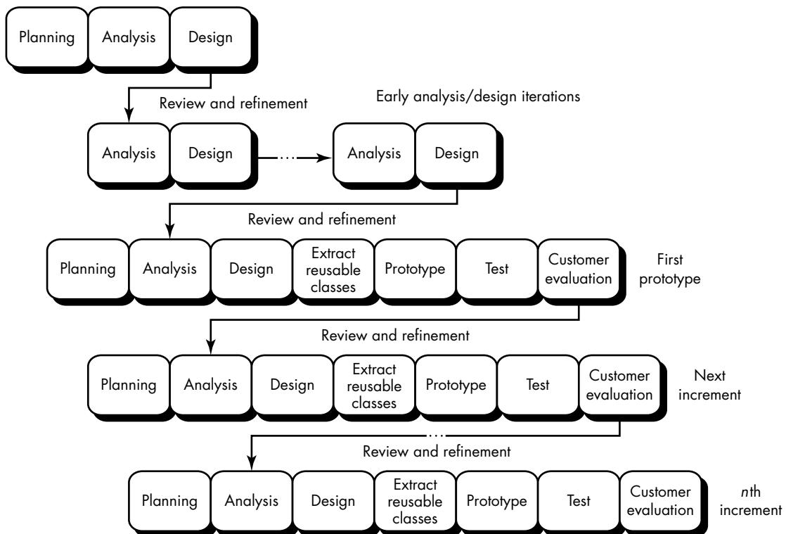
**FIGURE 20.11** Typical process sequence for an OO project
