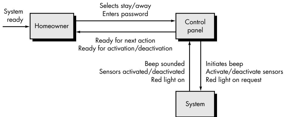
**FIGURE 21.11** A partial event flow diagram for SafeHome
