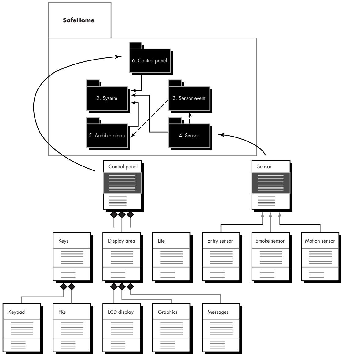
**FIGURE 21.7** An analysis model with package references
