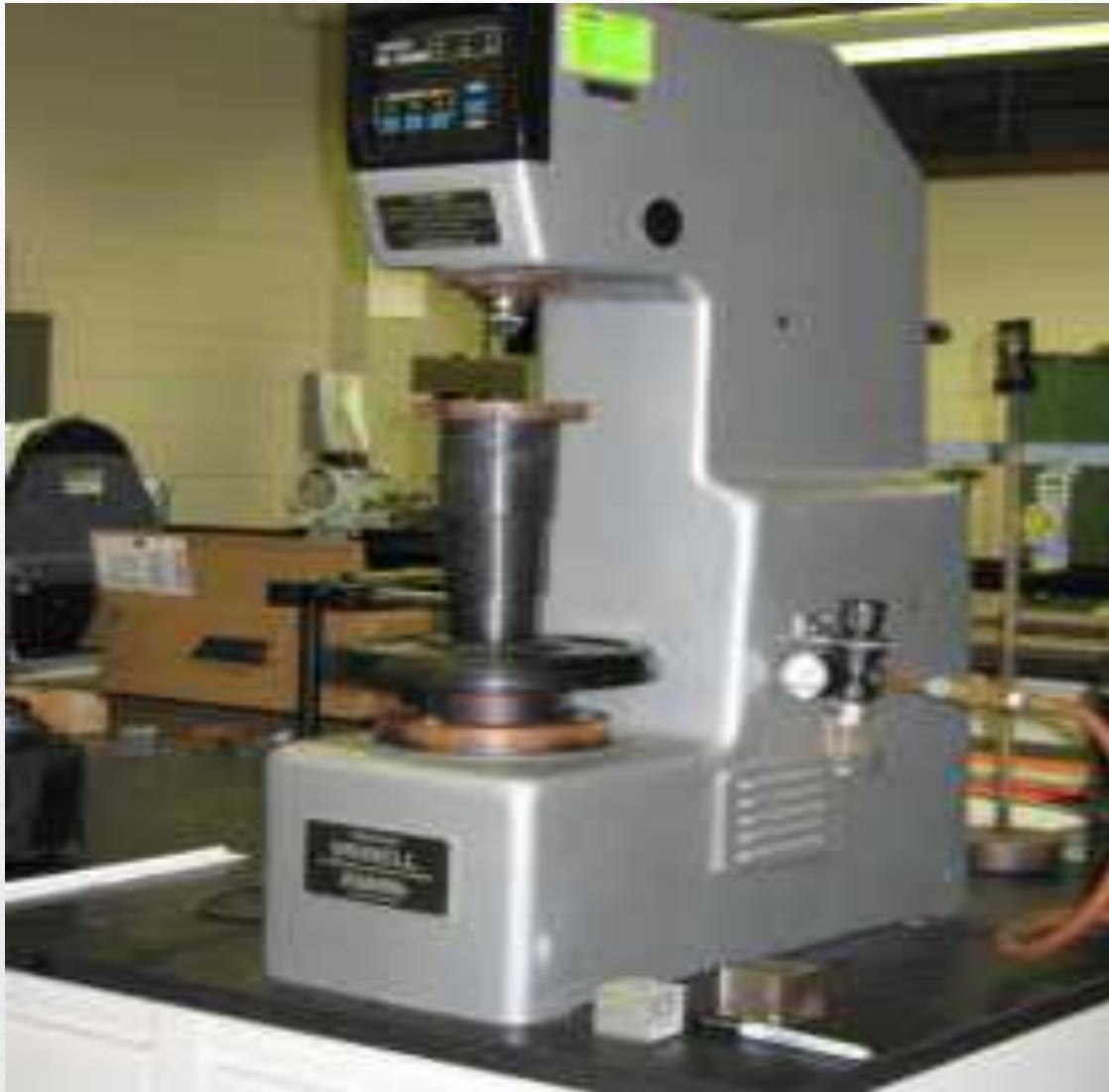
Figure 1 - Brinell Hardness Tester Model HB3000B
