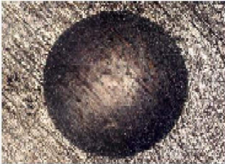
Impression on Brinell hardness test sample
