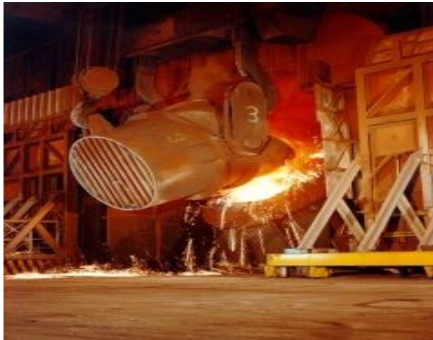
3) Charging hot metal to the BOS furnace
