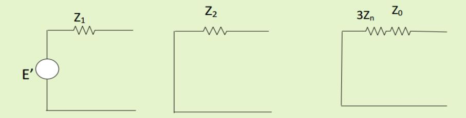
During a fault  $Z^1 \approx Z^2 \approx X_d^n$ . The zero sequence impedance is usually substantially smaller. The value of  $Z_n$  depends on whether the generator is grounded  Transformer Sequence Diagram
