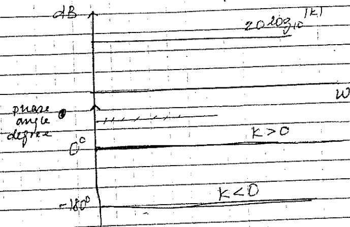
The effect of varying the gain  $K$  in transfer function is that it raises or lowers the log-magnitude curve of the transfer function.
