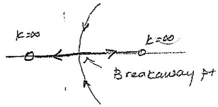
The breakaway point on the complete root loci of  $1+GH=0$  must
