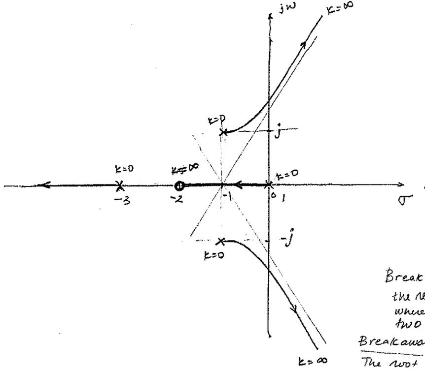
Break away pt - the pt where the root left the real axis. The locus leaves the real axis where there are a multiplicity of roots, typically two.
