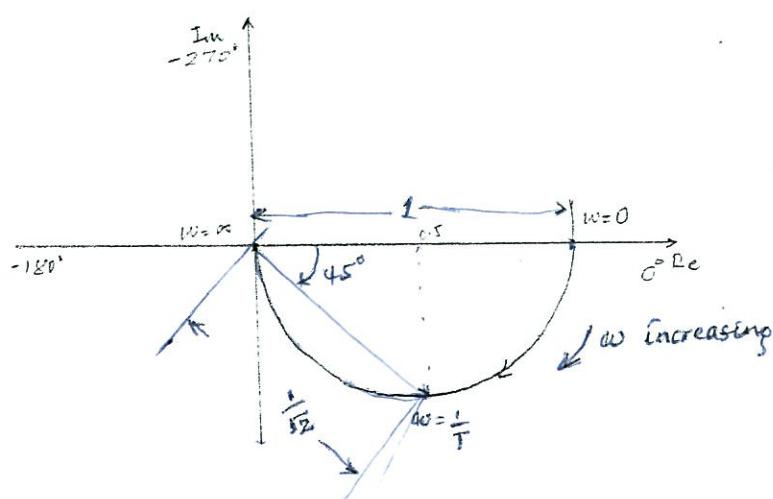
The polar plot is a semi-circle located at  $0.5$  on the real axis and radius  $\sqrt{2}/2$ .
