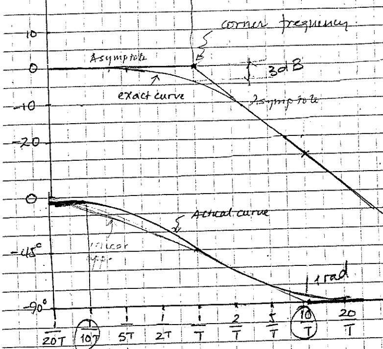
The frequency  $w = \frac{1}{T}$  at which the two asymptotes meet is called the corner frequency or the break frequency, which divides the plot into two regions, a low freq. region and a high freq. range.
