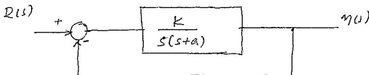
1- The closed loop transfer function  $T(s) = \frac{Y(s)}{R(s)} = \frac{GH}{1+GH} = \frac{K}{s^2 + as + K} = \frac{K}{s^2 + as + K}$
