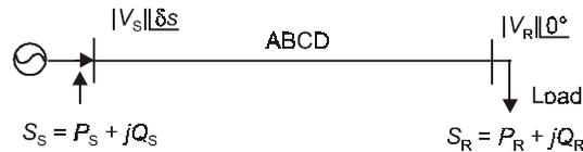
**Fig. 6.7:** Two bus sample power system.
