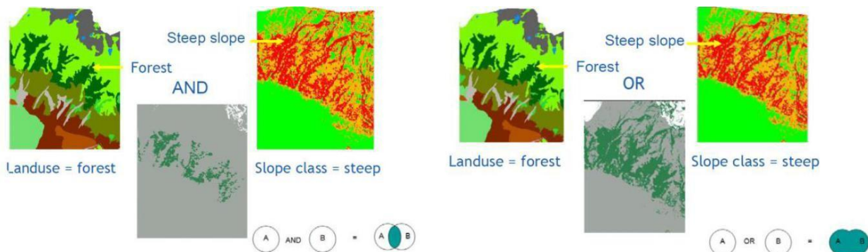
Overlay – logical operator AND
