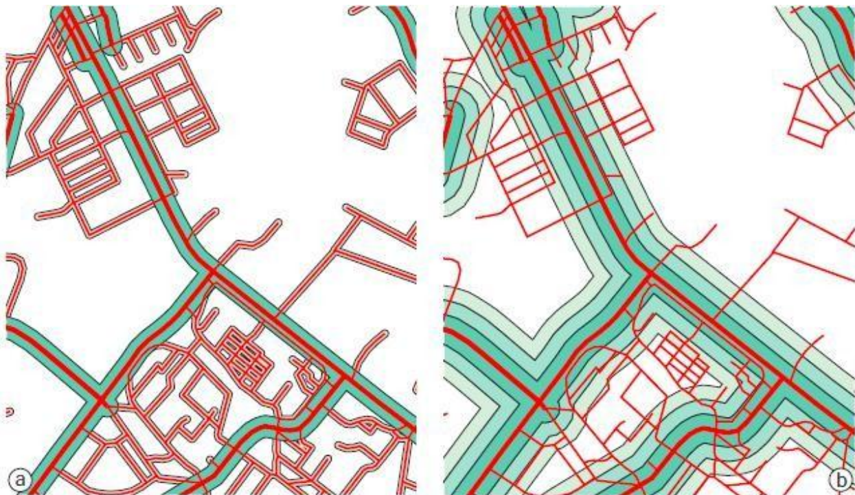
Figure 6-1: Buffer zone generation: (a) around main roads at 75m and around minor roads at 25m; and (b) Zonated buffers generated for three zones: at 100m, at 200m, and at 300 m of the main roads.
