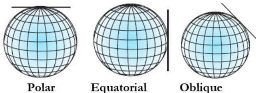
Figure 4-11: Azimuthal or planar projections
