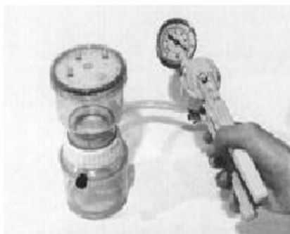
Fig.2.5. Using a manual vacuum pump to filter the sample through the membrane filter.
