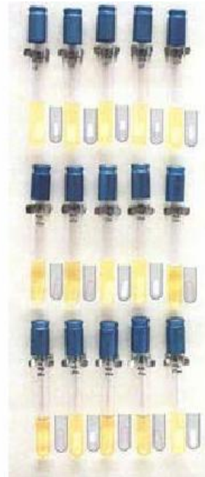
Fig. 2.13. Adding 1 ml of the 1:10 dilution to a test-tube 1:10 dilution of the sample.
