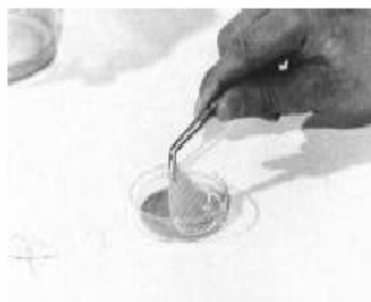
Fig.2.6. With a rolling action, placing the membrane filter on an absorbent pad saturated with membrane lauryl sulfate broth.
