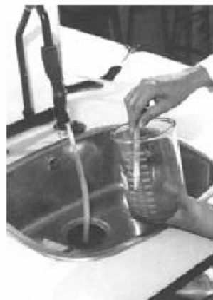
Fig.3.2. Removal of the supernatant with a suction pump
