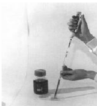
Fig 2.1. Adding 1.8 ml of sterile membrane lauryl sulfate broth to a Petri dish containing a sterile absorbent pad.
