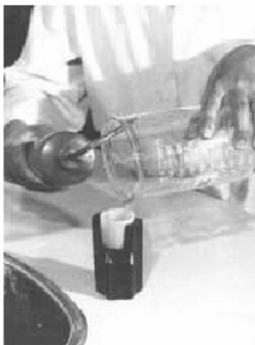
Fig.3. 3. Washing the sides of the container with dilute detergent solution.
