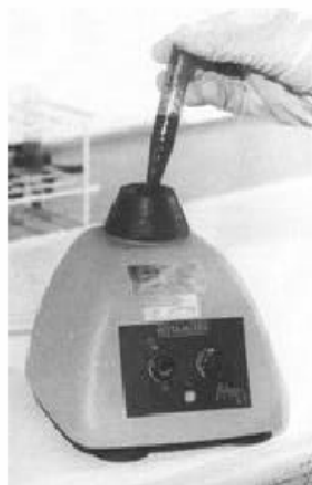
Fig.3. 5a. Homogenization of the sample can be carried out with a vortex mixer.
