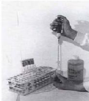
Fig. 2.12. Adding 1 ml of sample to 9 ml of diluent to make a containing 5 ml of medium A-1 and an inverted Durham tube.
