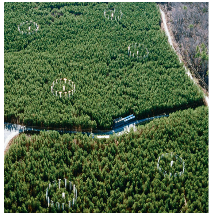
▲ Figure 56.28 Large-scale experiment on the effects of elevated CO 2 concentration. Rings of towers in the Duke University Experimental Forest emit enough carbon dioxide to raise and maintain CO 2 levels 200 ppm above present-day concentrations in half of the experimental plots.
