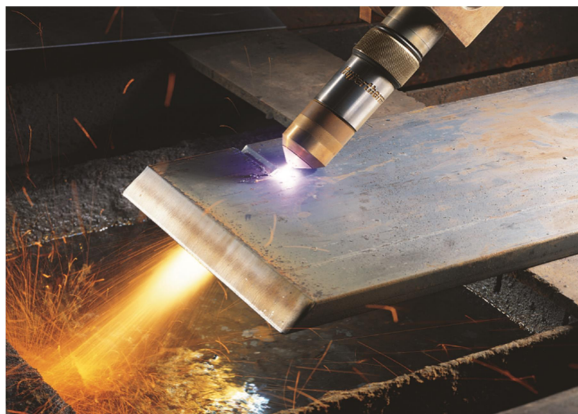
Figure 1.5: A plasma torch can be used to cut metal.
