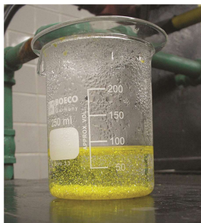
Figure 4.6: A precipitate of \text{PbI}_2 forms when solutions containing \text{Pb}^{2+} and \text{I}^- are mixed.
