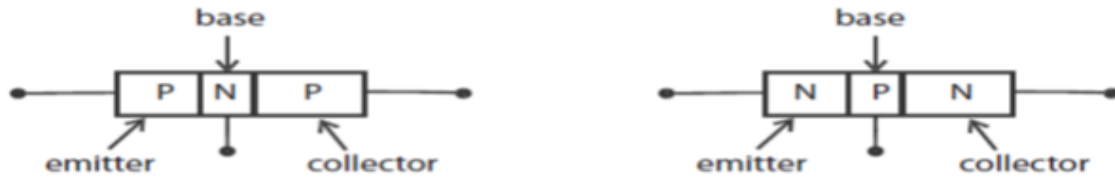
Figure 6.22: The two types of transistors, NPN and PNP.
