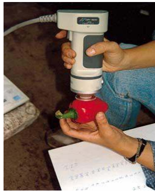
Fig. Objective colour measurement with a colourimeter
