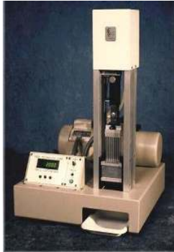
Fig. Tenderometer to test the pea maturity by presser tester
