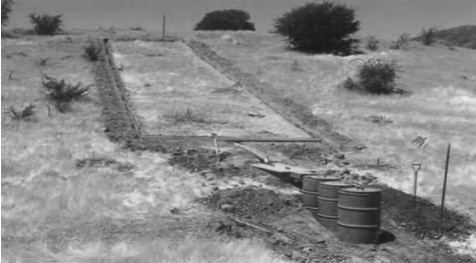
FIGURE 8.3. A plot to measure runoff and soil erosion
