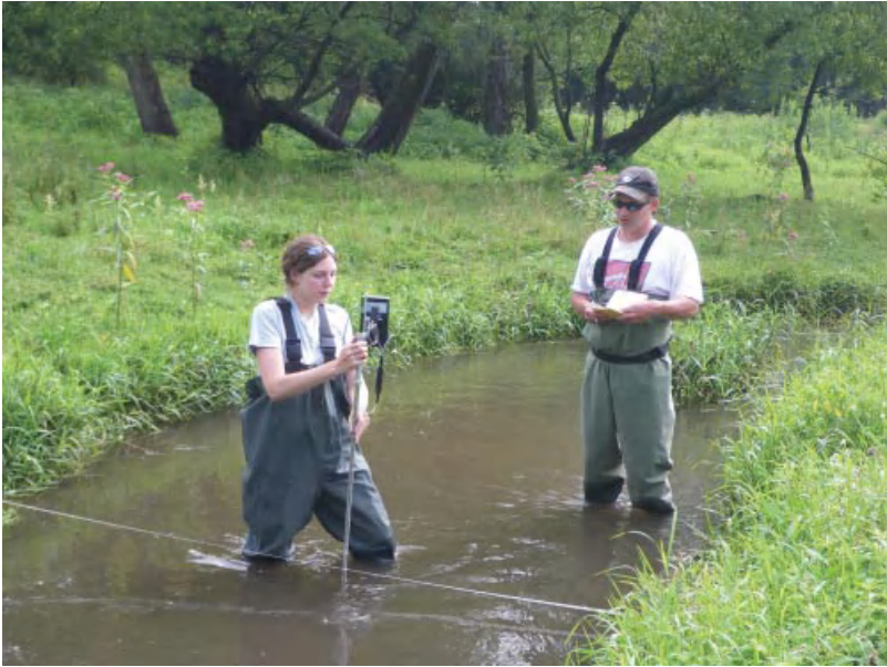
PLATE 3. Students measuring streamflow with a current meter (Photograph by Lucas Bistodeau)
