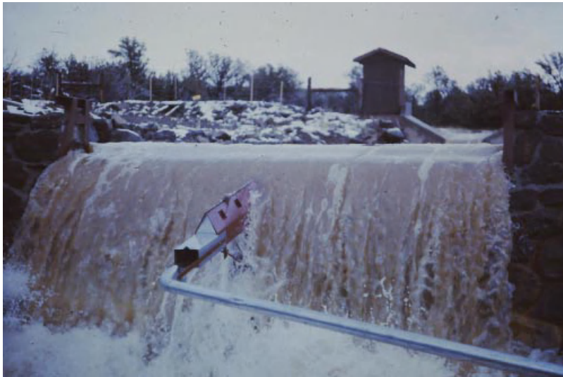
PLATE 7. A sediment splitter diverts progressively smaller fractions of streamflow to a collection tank to sample suspended sediment flowing through a rectangular weir in north-central Arizona. By also collecting bedload materials that settle in the catchment basin upstream of the weir total sediment yields can be measured from a watershed
