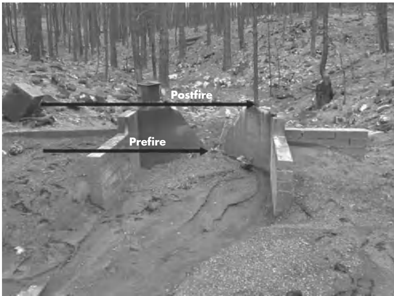
FIGURE 12.8. Streamflow discharge peak-flow stage shortly after cessation of the Rodeo-Chediski Wildfire in a ponderosa pine watershed in Arizona; prefire peak-discharge stage noted (For a color version of this photo, see the color plate section)
