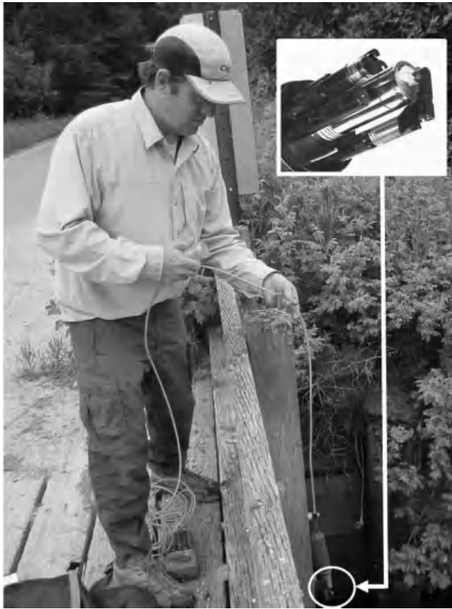
FIGURE 11.1. Measurement of DO with a multiparameter sonde (Photograph by Mark Davidson)
