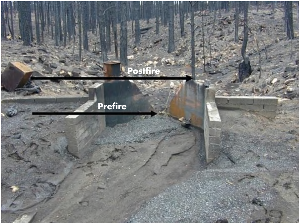
PLATE 11. Streamflow discharge peak-flow stage shortly after cessation of the Rodeo-Chediski Wildfire in a ponderosa pine watershed in Arizona; prefire peak-discharge stage noted
