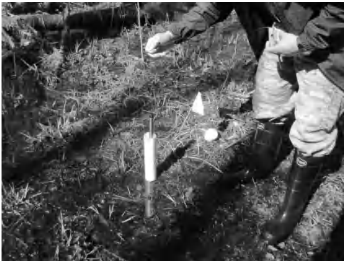
PHOTO 1. Measuring groundwater levels in a forested wetland with a pressure transducer in a shallow well (Photograph by Chris Lenhart) (For a color version of this photo, see the color plate section)
